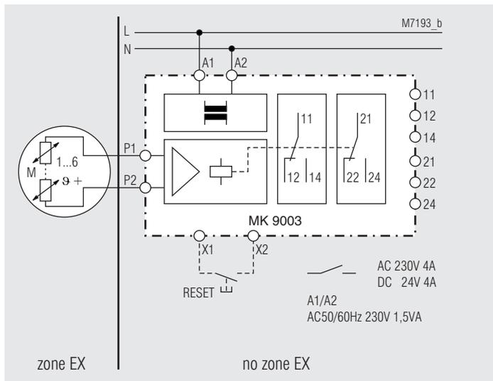
Thermistor motor protection relay shown as variant MK 9003/\_1\_ \_ \_ , with safe separation according to EN 61 140, EN 60 947-1, 6 kV/2 between:
