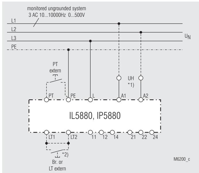
Monitoring of an ungrounded voltage system.
