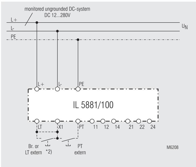
Monitoring of an ungrounded system without auxiliary supply.
