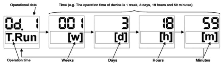
All operational data is deleted by pressing "Mode" and "Test" for more than 2 seconds in operational data display mode. The reset is confirmed on the display "ResOd" (Reset operational data).
