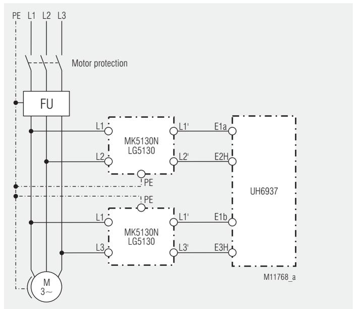
Inverter monitoring function, 3-phase with frequency monitor UH 6937
