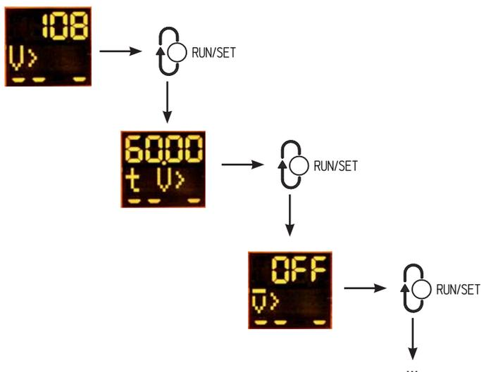
The default values set in the parameters (see parameter table) can be individually adjusted with the ▼▲ buttons; however, they must be within the respective setting ranges. The next parameter can be selected with the RUN/SET button and also be adjusted with the ▼▲ buttons.
