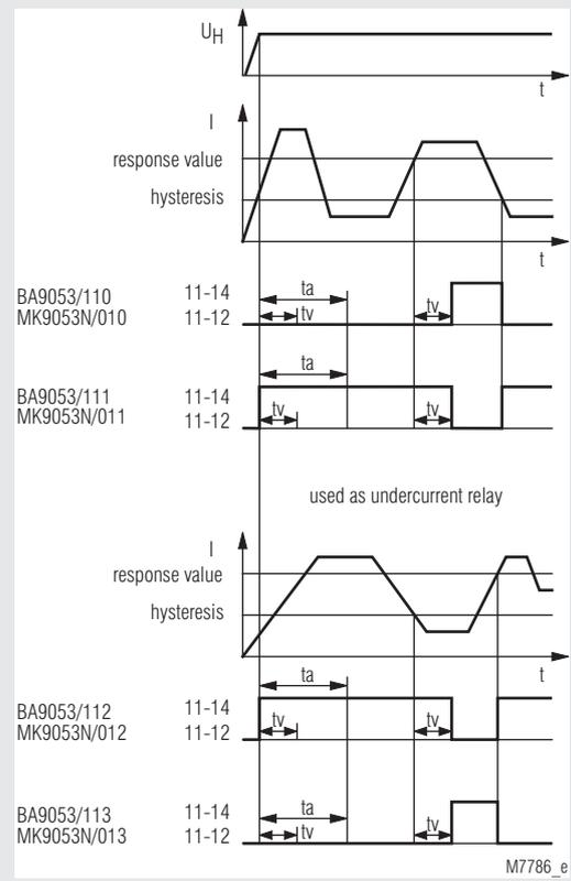
On model BA 9053/6\_\_ with manual reset the contacts remain in the fault state after detecting a fault or after  $t_o$  has elapsed. The contacts are reset by disconnecting the supply voltage.
