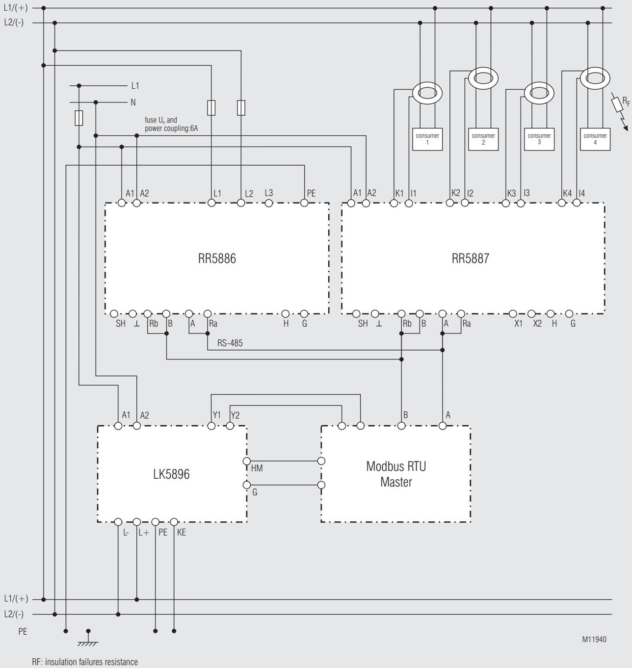
Insulation fault location via Modbus control with external master.
