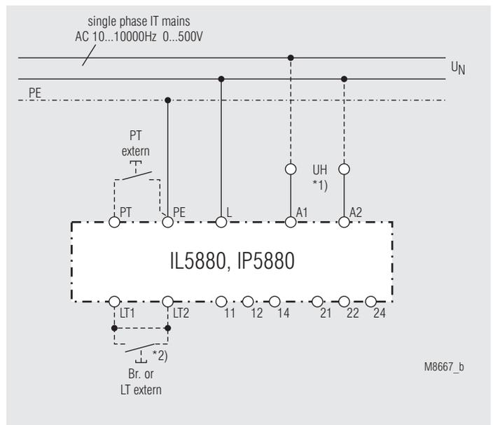
Monitoring of an ungrounded voltage system.
