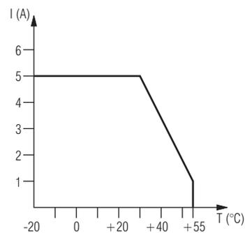
continuous current limit curve (current over 2 contacts) M8367
