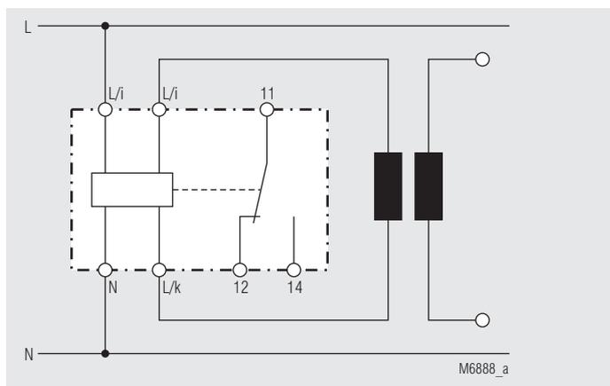
Connection Example with external galvanical separation, e.g. via current transformer.
