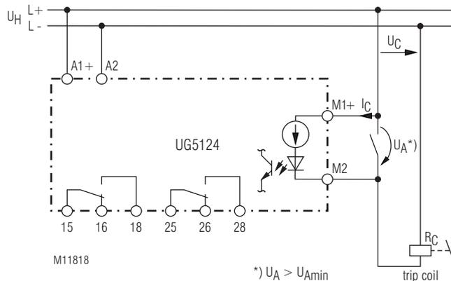
The voltage  $U_{Amin}$  has a hysteresis of 2%. I.e. the relay switches at a voltage of  $U_{Amin}$  - Hysteresis in error state (contacts 15, 16 and 25, 26 closed). If the voltage  $U_{Amin}$  is acceded, the relay switches to good stated (contacts 15, 18 and 25, 28 closed).
