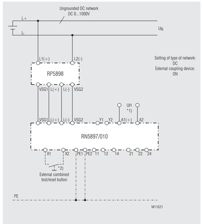
\*1) Auxiliary voltage  $U_H$  (A1(+)/A2) ) can also be sourced from the monitored voltage system.
