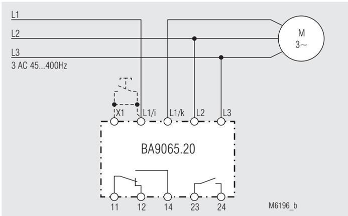
Without current transformer ( $I_{Mot} = 0.5 \dots 10 \text{ A}$ )
