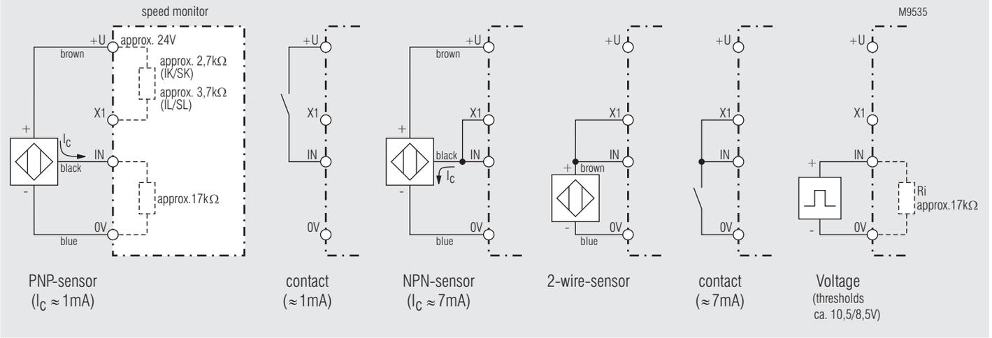
Note: For IK-models the auxiliary voltage (DC 24 V) must be additionally connected to terminals +U/0V
