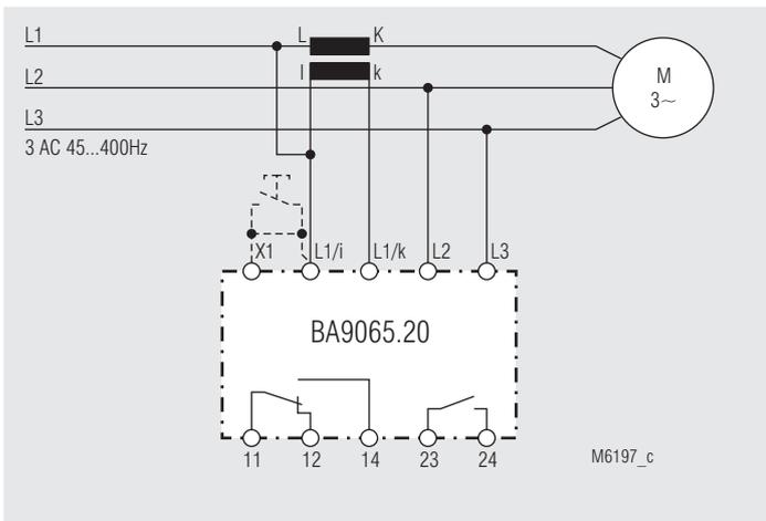
With current transformer ( $I_{Mot} > 10 \text{ A}$ )
