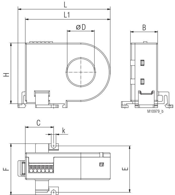
for DIN rail mounting or screw mounting
