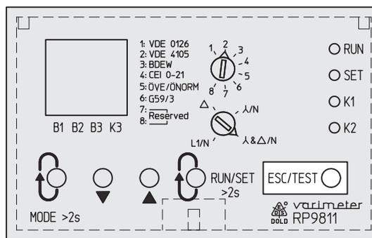
Wrong or contradictory entries of parameter values are recognised and displayed by the device as errors (setup errors). The error status can be exited by pressing the RUN/SET button longer than two seconds. The faulty parameters can be corrected back in the input mode.
