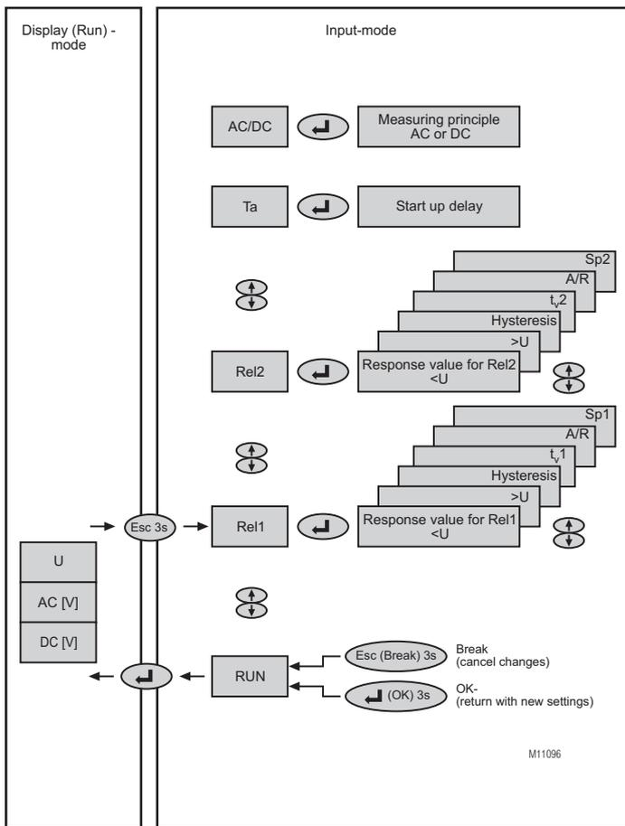
After connecting the auxiliary supply A1/A2 the unit is in display (Run) mode:
