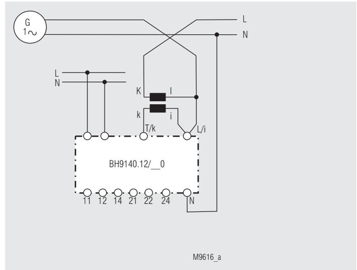
For single or 3-phase connections with current transformer (external)
