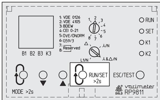
To change the parameters manually, the RUN/SET button must be pressed longer than two seconds. The display mode is accessed. The input mode is accessed when subsequently pressing "▼▲". The input mode is also accessed by turning one of the two rotary switches.
