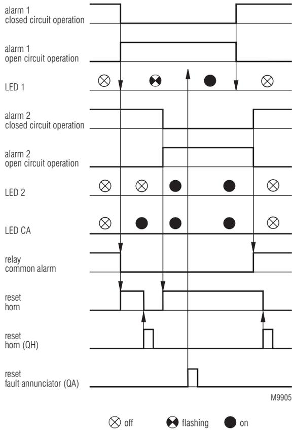
**Function Diagram (Common Alarm Annunciator, Auto Reset)**
