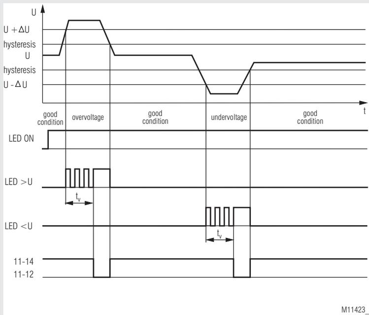
Monitoring function: voltage range; rotary switch: „U<>“
