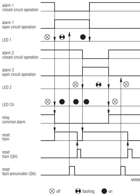
**Function Diagram (Common Alarm Annunciator Manual Reset)**
