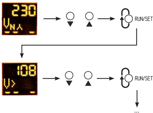
After the desired changes have been made, the new values are saved by pressing the RUN/SET button (> 2 s).
