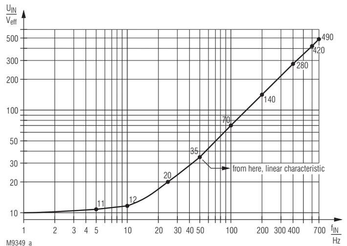
Typical sensitivity of the measuring input at variant
