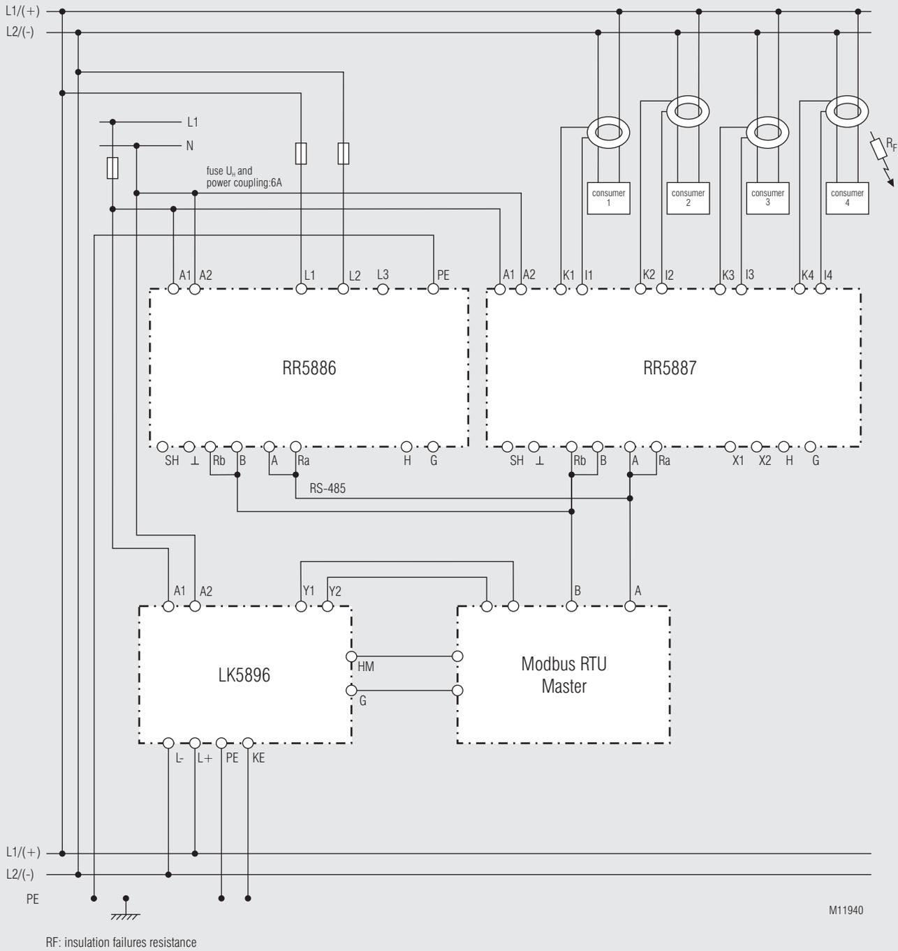
Modbus control insulation fault detection with external bus master
