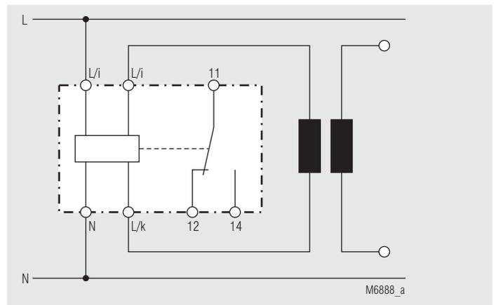
Connection Example with external galvanic separation, e.g. by current transformer
