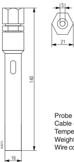
Probe made of stainless steel,
