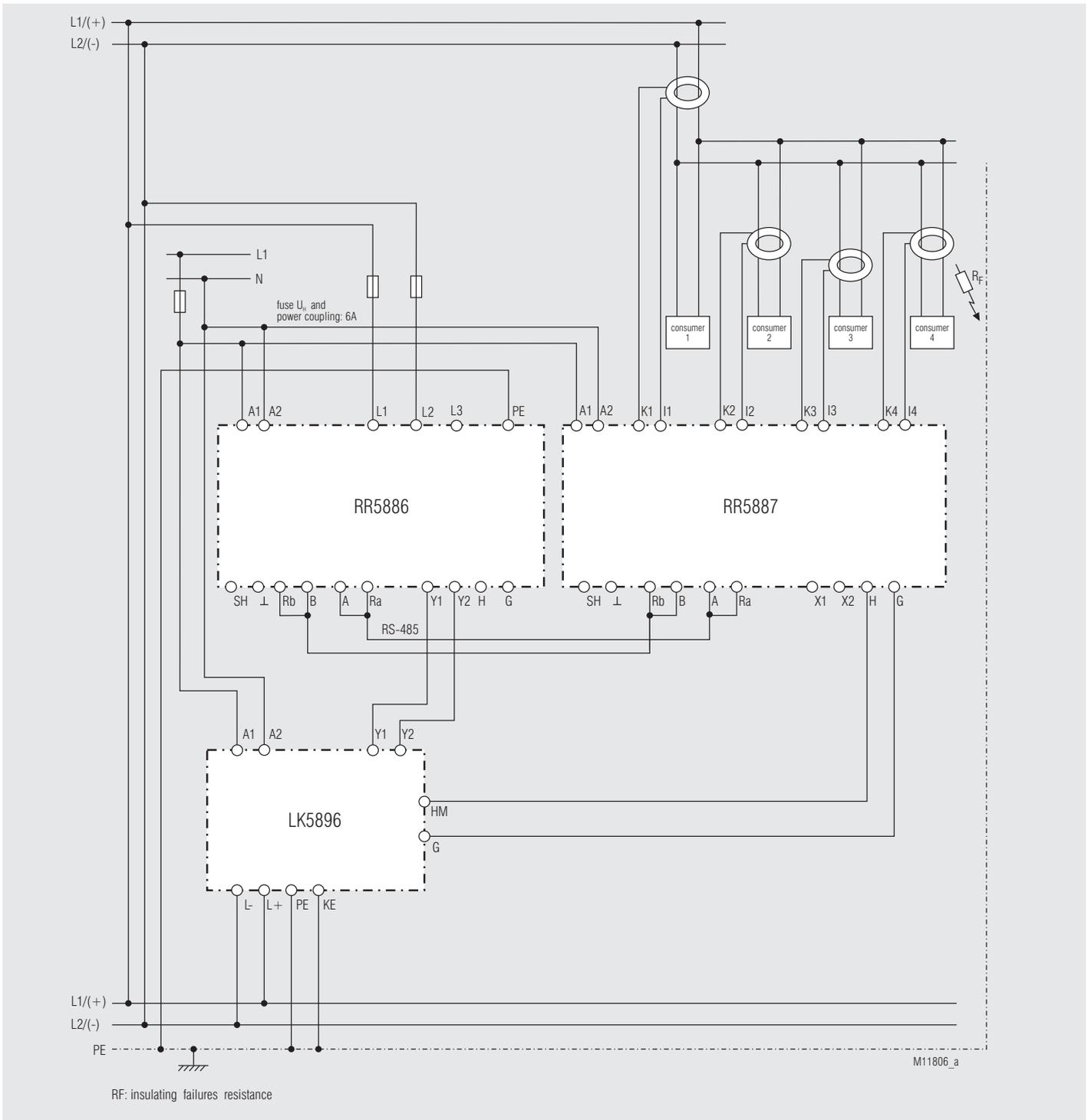
Insulation monitoring and insulation fault detection with 4 connected measuring current transformers in a AC (DC)- network with subdistribution - insulation fault detection can be controlled by the insulation monitor /LK 5896); ALARM MEMORY active, i.e. alarm states are stored; bus termination of the first and last device on the RS-485 bus.
