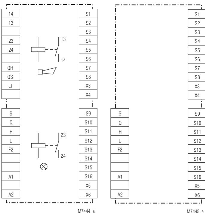
On EP 5966 and 5967 open circuit operation or closed circuit operation can be selected by bridging terminals X3/X4 or X5/X6 for 2 groups of 8 inputs. To avoid unnecessary fault signalling an operate delay of 1 s, 3 s or 10 s to the inputs is available.
