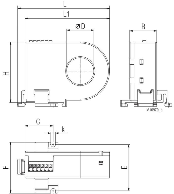
for DIN rail mounting or screw mounting
