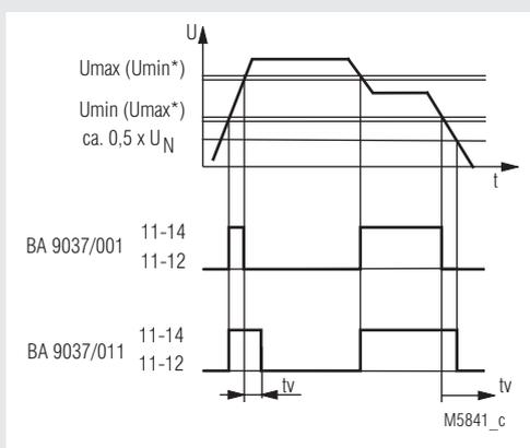
\*  $U_{min}$  and  $U_{max}$  can also be exchanged. The hysteresis of the setting values is  $< 4\%$  of the response value
