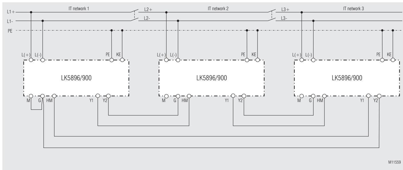
Monitoring of 3 separate DC voltage systems, that can be coupled by coupling switches. By sequential triggering of the insulation monitors it is made sure that only one of the insulation monitor is active at the same time. the first insulation monitor in IT network 1 is configured as master and starts the measuring cycle after power up.
