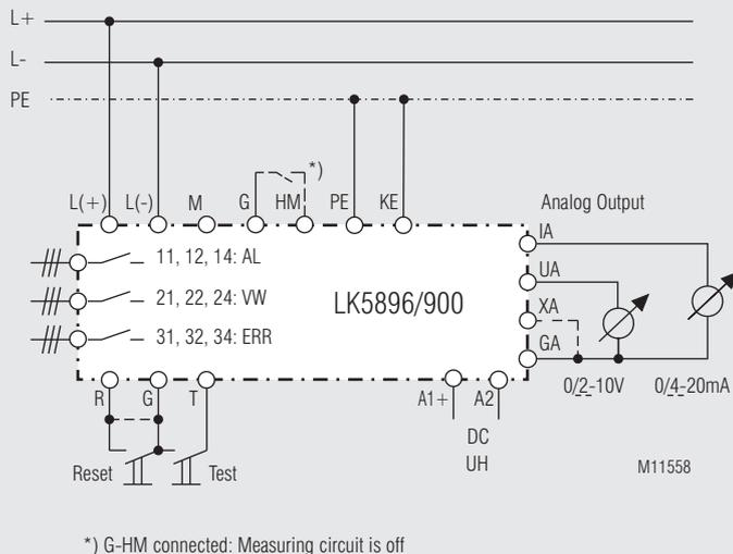
Connection to a simple DC system. When terminals HM-G are open the device triggers itself automatically.
