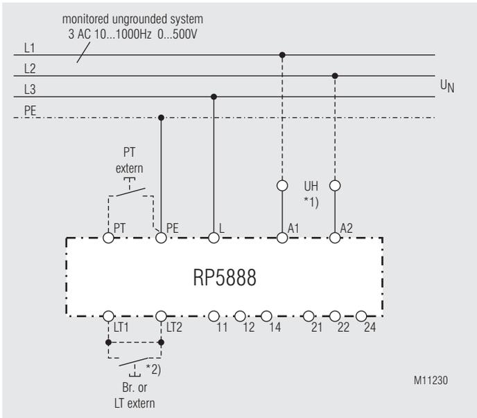
Monitoring of an ungrounded voltage system.
