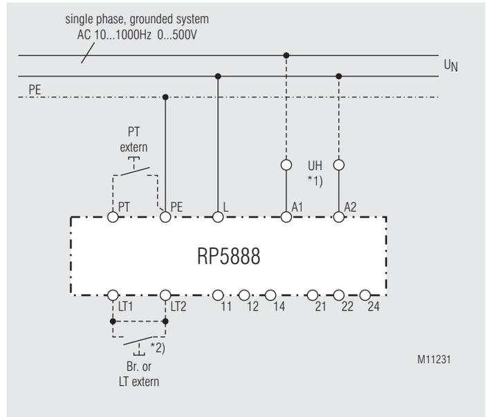
Monitoring of an ungrounded voltage system.
