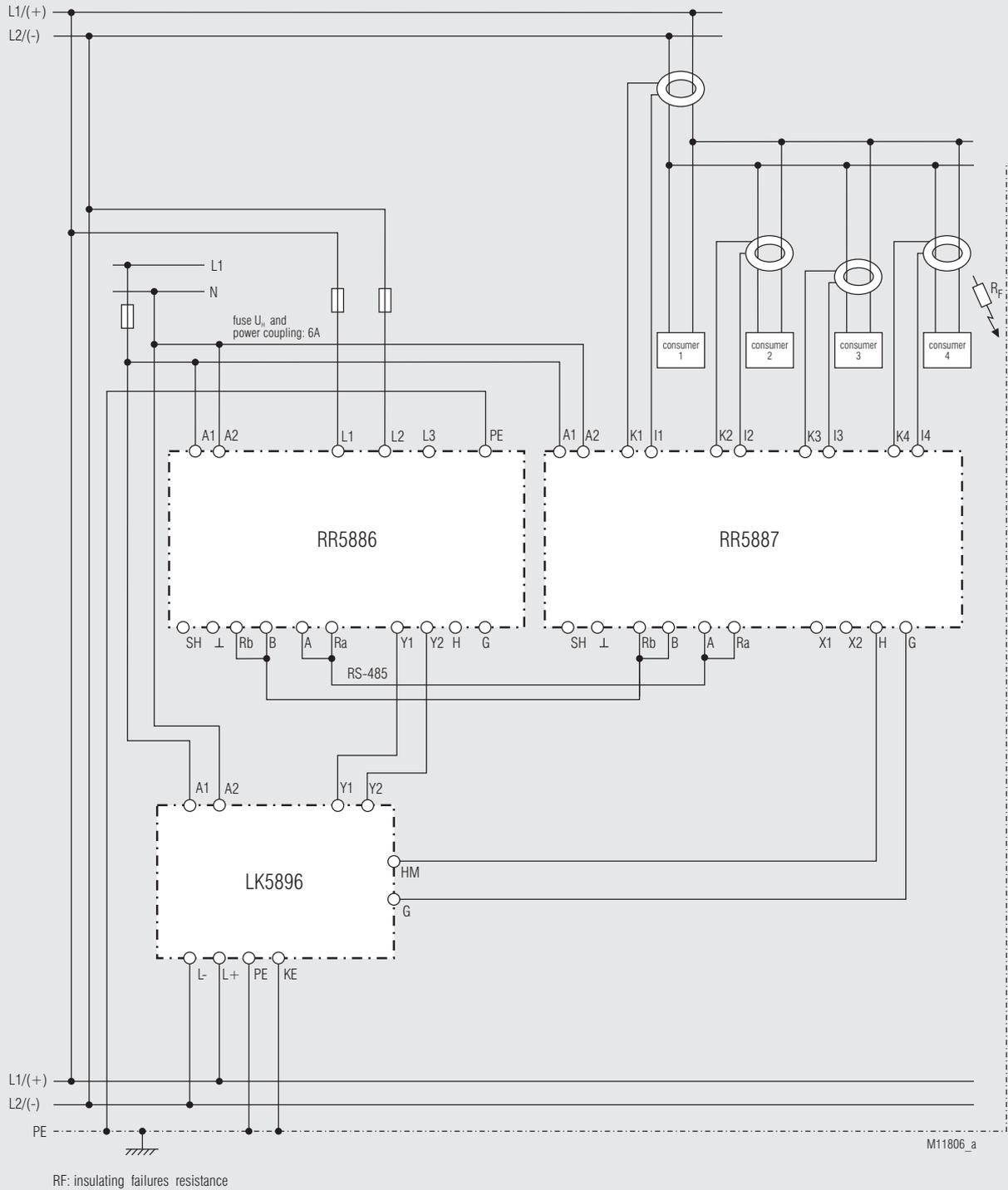
Insulation monitoring and insulation fault detection with 4 connected current transformers in a AC (DC)- network with subdistribution - insulation fault detection can be controlled by the insulation monitor /LK 5896); ALARM MEMORY active, i.e. alarm states are stored; bus termination of the first and last device on the RS-485 bus.
