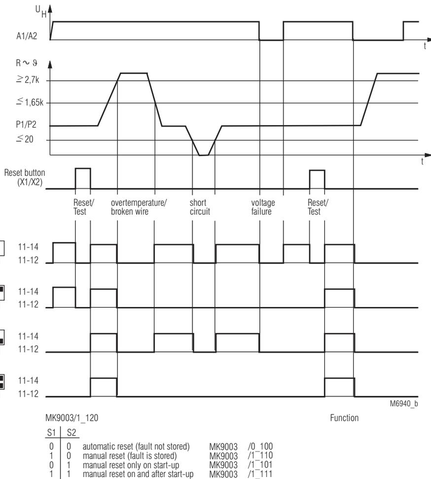
**With manual reset, also after voltage failure (no start-up reset)**
