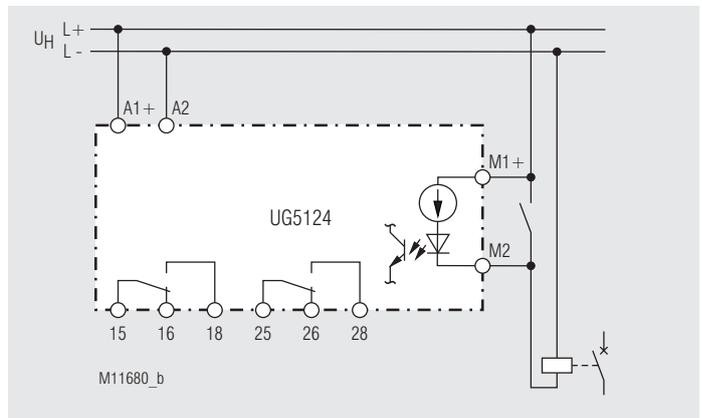
Auxiliary voltage / measuring voltage separate connection or common connection to one voltage source.
