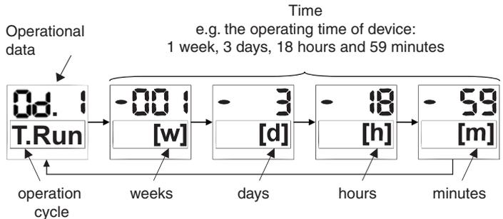
All operational data is deleted by pressing "Mode" and "Test" for more than 2 seconds in operational data display mode. The reset is confirmed on the display "ResOd" (Reset operational data).
