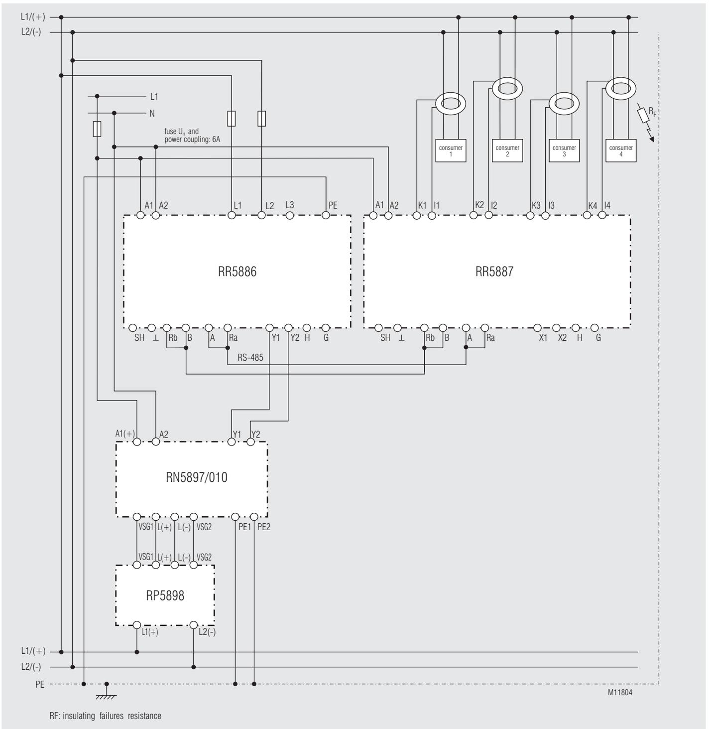
Insulation monitoring and insulation fault detection with 4 connected current transformers in a AC (DC)- network with subdistribution - insulation fault detection can be controlled by the insulation monitor (RN 5897/010); bus termination of the first and last device on the RS-485 bus.
