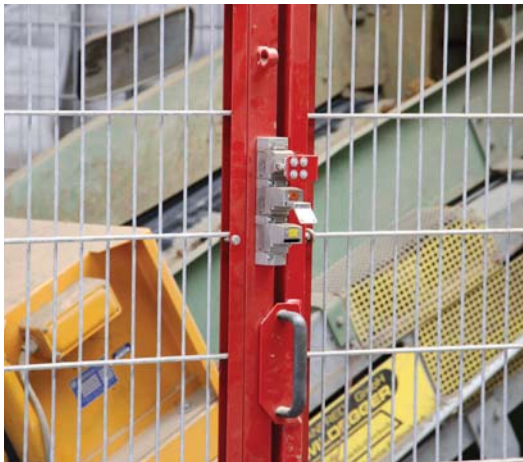
The purely mechanical guard locks at the doors consist of stainless steel and are therefore extremely robust.
